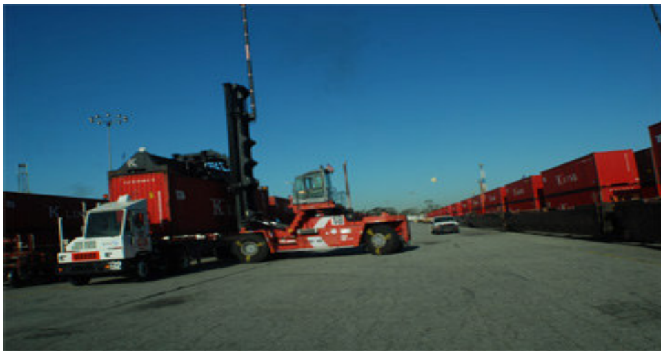
Figure 6 Toploader from double stacked train to bombcart
