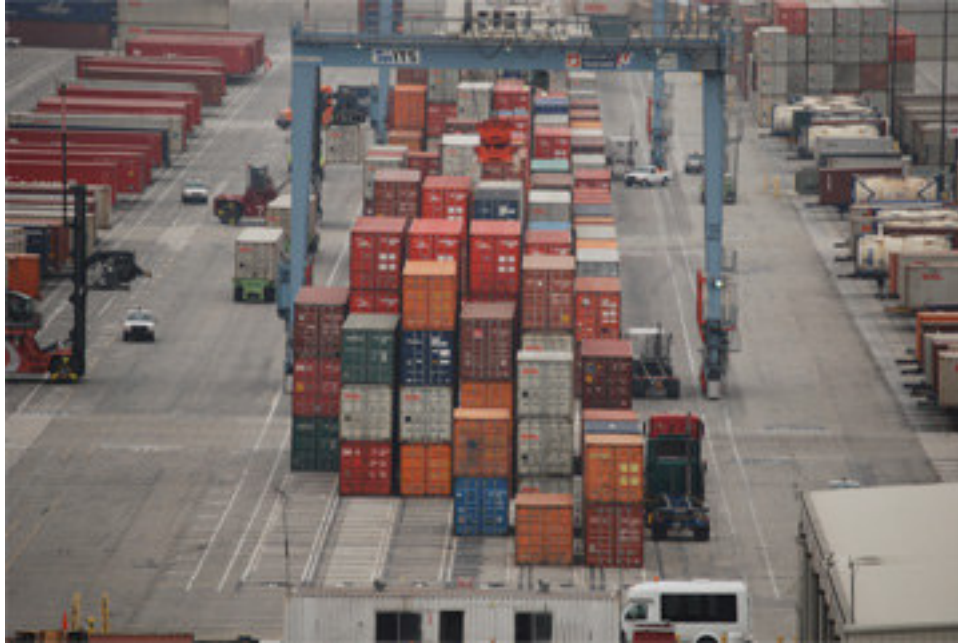
Figure 2 Tire gantry crane to drayage truck from storage
