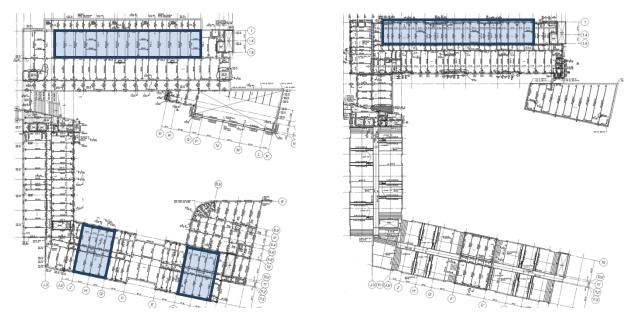
Figure 3: 2<sup>nd</sup> Floor (left) and 3<sup>rd</sup> Floor (right) framing plans. Typical bays on each level highlighted. Courtesy of RIT. Drawings not to scale.
