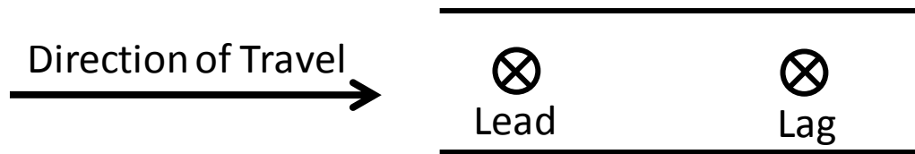
Figure 1.1: Sensors in a speed trap configuration with the lead sensor and lag sensor 14 ft to 22 ft apart
