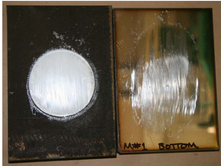
Figure 4-1. mirror polished specimen after test M1.45.250.100
