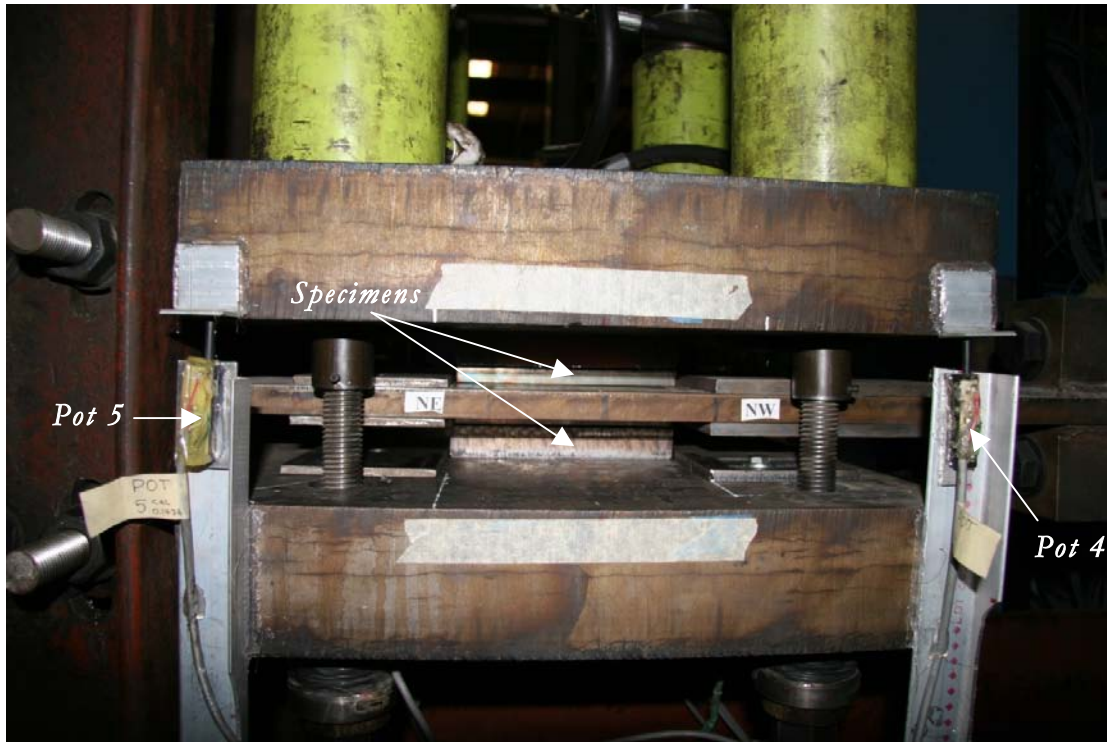
Figure 3-7. Showing the specimen carriers and pots 4 and 5
