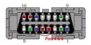
Figure 8.2 – Pins 4 and 5 of the J1962 DLC
