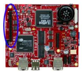
Figure 3.8 – The JTAG connector highlighted on the TS-7390 SBC
