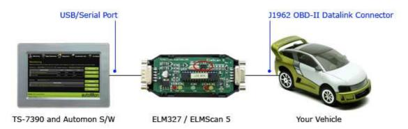
Figure 4.1 – How Automon Connects to Various Components
