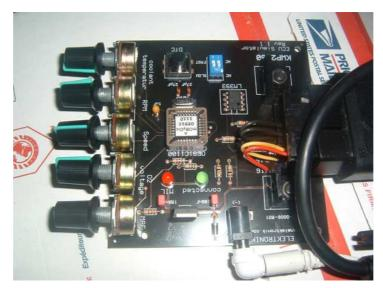
Figure 3.13 – The KWP2000 EOBD ECU Simulator in the development of Automon
