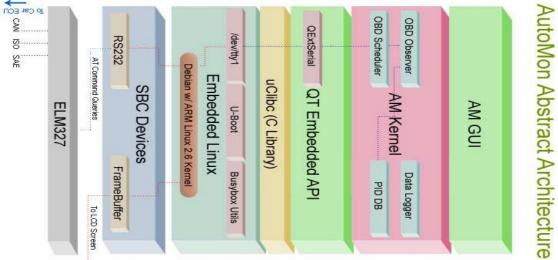
Figure 4.2 – High Level Software Architecture
