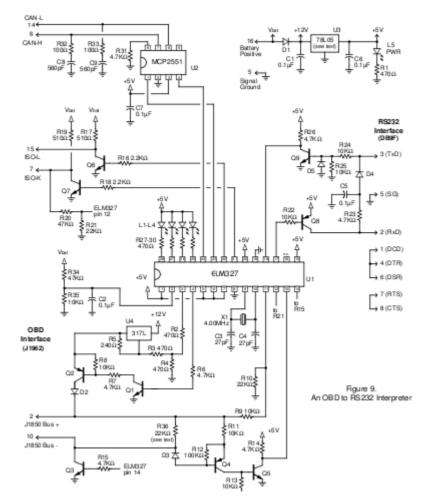
Figure 3.10 – A Recommended Circuit for the ELM327
