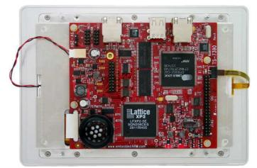
Figure 3.7 – The TS-7390 SBC at the back powering the device
