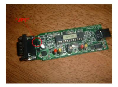
Figure 8.3 – ElmScan 5 and the jumper to change to join pins 4 and 5. The ELM327 can also be seen
