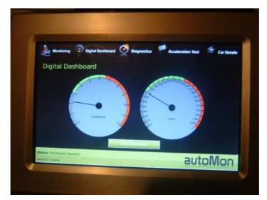
Figure 1.1 – Automon running on the single board computer (SBC)
