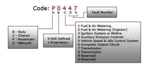
Figure 3.5 – Example of a Diagnostic Trouble Code
