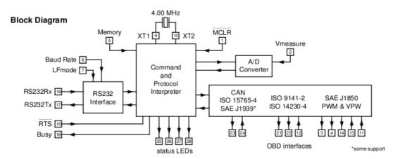
Figure 3.9 – Block diagram of the ELM327 Integrated Circuit
