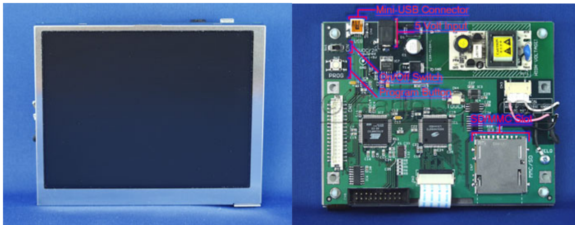
Figure 6. ezLCD-004 Touch Screen/Microcontroller Kit
