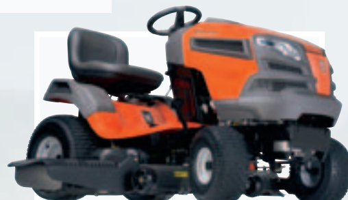
Cast iron front axle and welded chassis add strength and stability.
