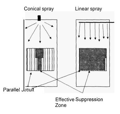
Figure 1. Zones of effective fire suppression in arrays of printed circuit boards, using conical and linear sprays.
