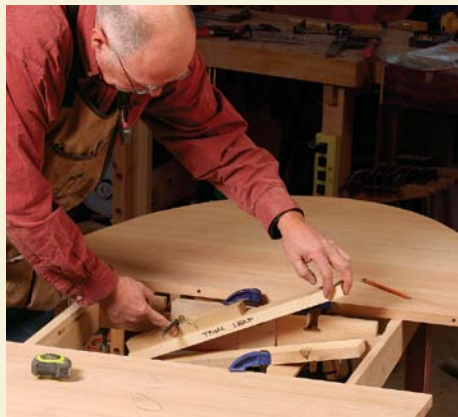
Put a temporary leaf in place. Fortune clamps a piece of plywood with a pivot hole to the cross-stretcher. He then puts a transfer punch (or drill bit) in place of the window bolt.
