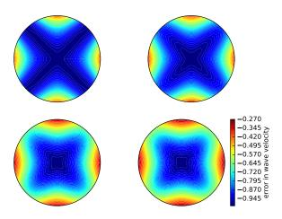
Figure 7: Error in numerical dispersion in 2D
