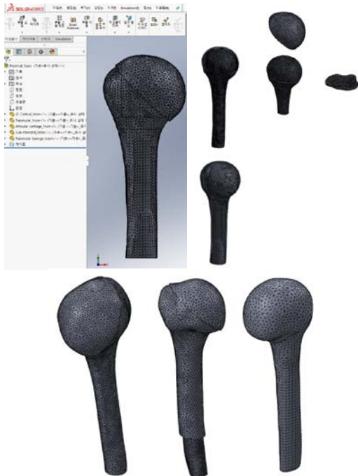
Figure 5. 3D modeling of four reconstructed structures of the humerus (cortical bone, trabecular bone, articular cartilage, sub-chondral) with SolidWorks 2017.
