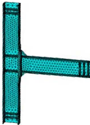
Fig. 3 – A typical finite element model of connections.
