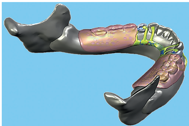
Figure 4. Multiple solid parts (implants, IARPD metal framework parts, IARPD acrylic resin structures, and attachments components) positioned as one entity in relation to mandibular model (exported as Parasolid XT file). IARPD, implant-assisted removable partial denture.
