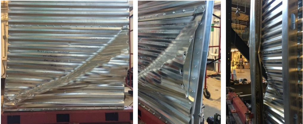
(a) Sheet buckling (b) Screw pulling over (c) Stud buckling
