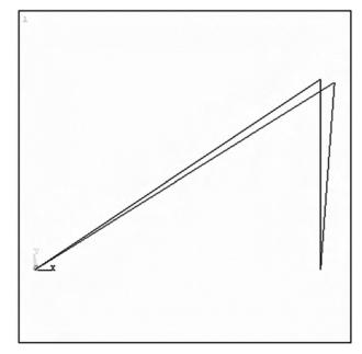
In general, the displacements are relatively small. Thus, most graphical postprocessors amplify the displacement so that the deformed shape of the truss can be shown in the figure.
