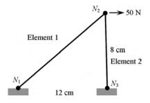
Figure C.3 Two-bar truss
