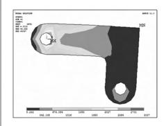
The colors in the contour plot stand for the level of von Mises stress. The maximum stress occurs at the fixed pin hole. The value of stress can be read from the color legend in the bottom of the graphic screen. Note that the color legend can be shown on the right side of graphic screen. You can also produce an animated version of these results:
