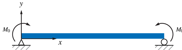
Figure 4.2: Simply supported beam subject to bending moments
