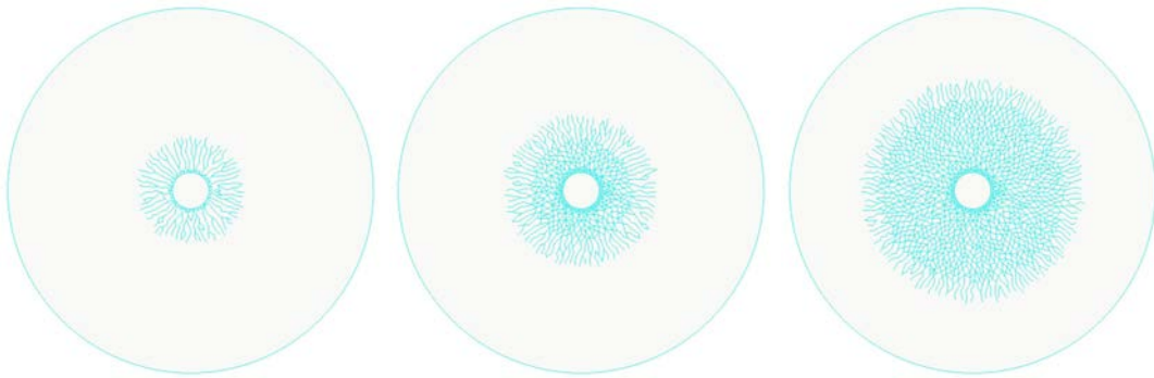
Figure 9: Fracture of brittle disk under core expansion.
