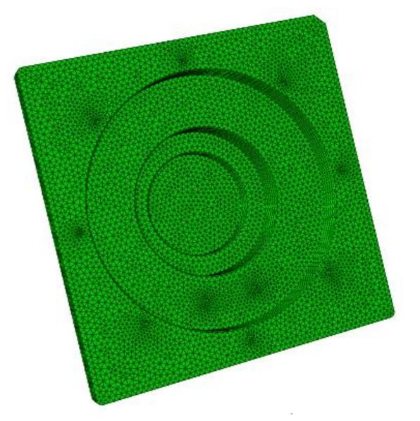
Hollow underside reduces mass of standard: makes it easier to work with
