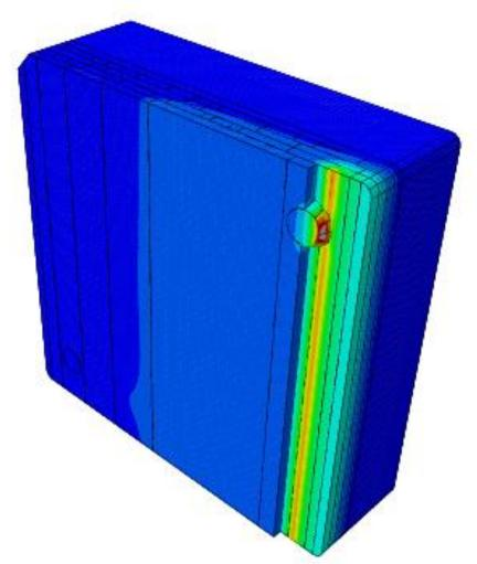
Region at a temperature above ambient does not go very far into the material.
