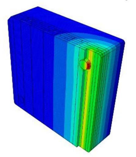
Region at a temperature above ambient goes much further into the material.
