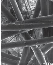
Right: This outer layer of the 7CVP consists of a dense matrix of glass fibers. The coalescing outer layer provides highly efficient aerosol removal with very low pressure drop.
