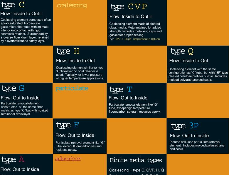
Hydrocarbon vapor removal element. Ultrafine grained, highly concentrated, activated carbon sheet media. Includes molded polyurethane end seals. Particulate = type G, T, F, 3P Adsorber = type A
