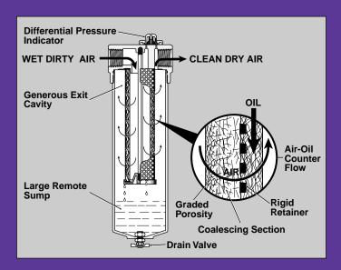
This coalescing filter depicts bow the air flows from the inside out. This bousing contains a coalescer with a built in prefilter.
