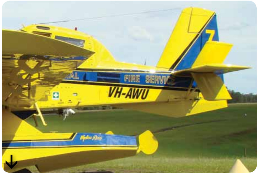
Plate 12. View of ventral fin, the sealed fuselage/stabilizer, top vertical fin and the fairing over the open fuselage structure near the landplane tail-wheel mount and the retractable steering water rudders.
