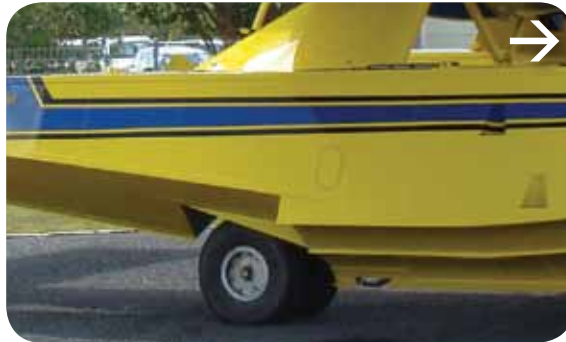
Plate 15. Shows the location of scoop which is forward of the wheeled landing gear.
