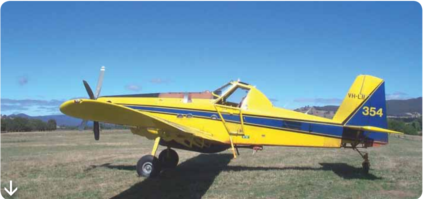
Plate 25. Bomber 354 (Delatite, VIC) a standard one seat Air Tractor AT-802AF fitted with a conventional undercarriage, Air Tractor FRDS and a PT6A-65A fitted with a 1295-shp turboprop engine.
