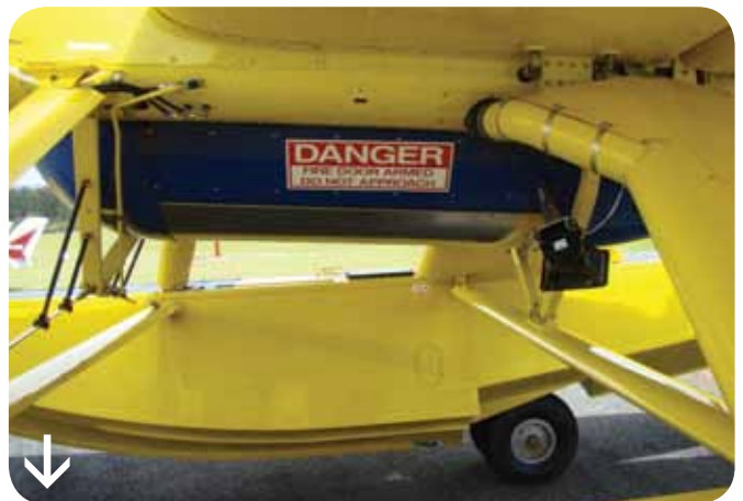
Figure 1. Both images show the standard Air Tractor FRDS and the location of the fuselage supports for the amphibious floats which appear to offer no interference to the drop evacuation process.
