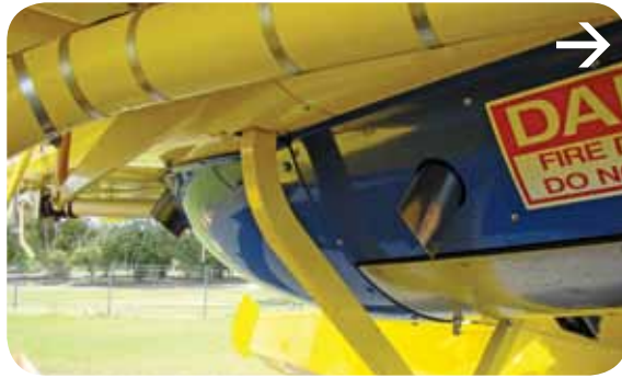
Plate 19. Shows the original 75 millimetre and new 125 millimetre fire gate venting.
