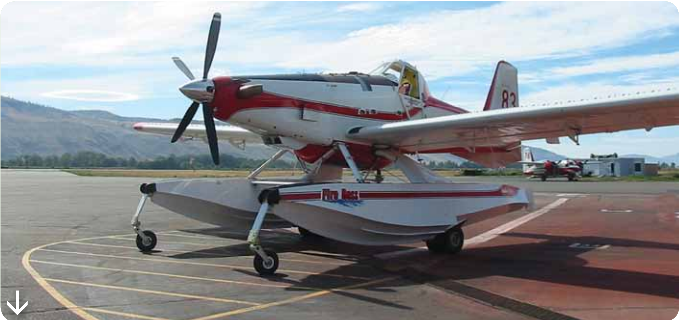
Plate 27. Tanker 83 (Kamloops B.C. Canada) a one seat Fire Boss Air Tractor AT-802AF fitted with the Wipline amphibious undercarriage with subsequent airframe modifications, Air Tractor FRDS and fitted with a PT6A-67AG fitted with a 1350-shp turboprop engine.
