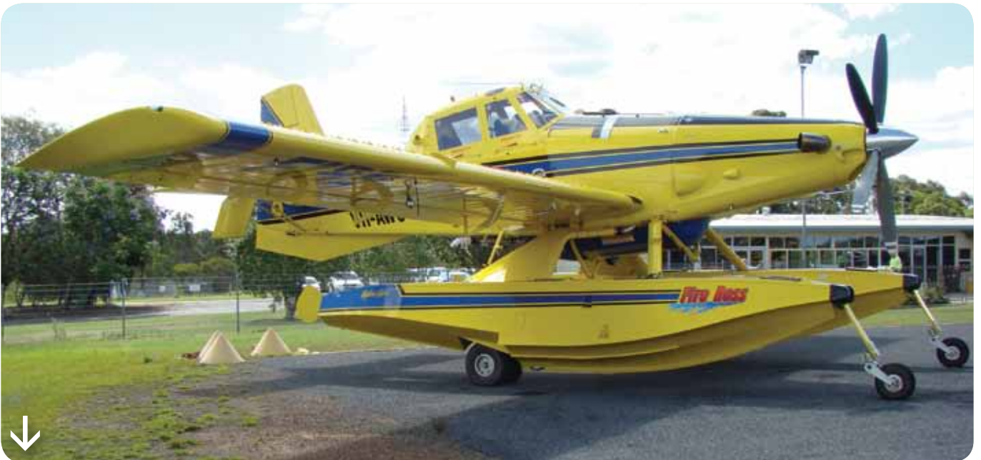
Plate 28. Bomber 718 ( Grafton, NSW) a two seat Fire Boss Air Tractor AT-802F fitted with the Wipline amphibious undercarriage, Air Tractor FRDS with subsequent airframe modifications and fitted with a PT6-67F 1600-shp turboprop engine.
