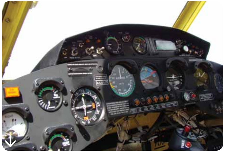
Plate 22. Additional upper instrument bank, to monitor landing gear, manage scooping operations, including payload management.
