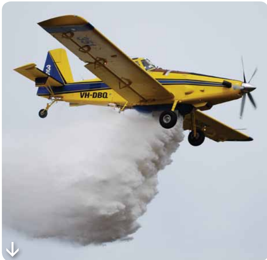
Plate 8. Bomber 351, AT-802F (Stawell, VIC) delivering a full salvo of water injected with foam concentrate.
