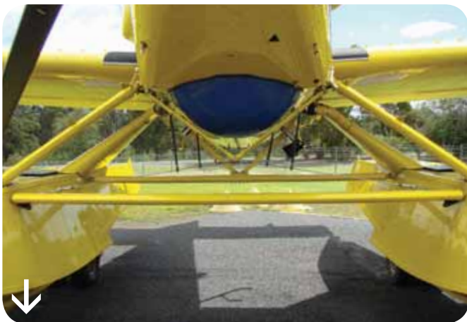
Figure 1. Both images show the standard Air Tractor FRDS and the location of the fuselage supports for the amphibious floats which appear to offer no interference to the drop evacuation process.
