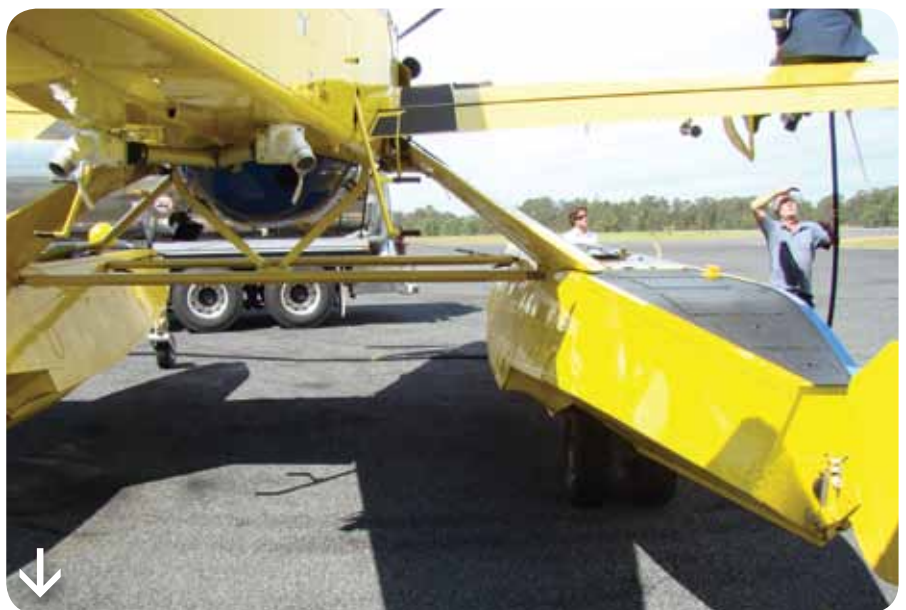
Plate 24. Refuelling operation for the Fire Boss, indicating the height perspective and showing also the height of the reloading ports under the fuselage.
