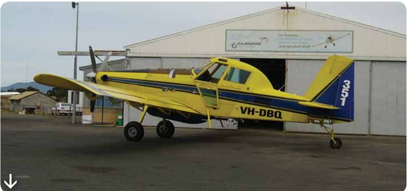
Plate 26. Bomber 351 (Stawell, Vic) a standard two seat Air Tractor AT-802F fitted with a conventional undercarriage, Air Tractor FRDS and a PT6A-67AG fitted with a 1350-shp turboprop engine.
