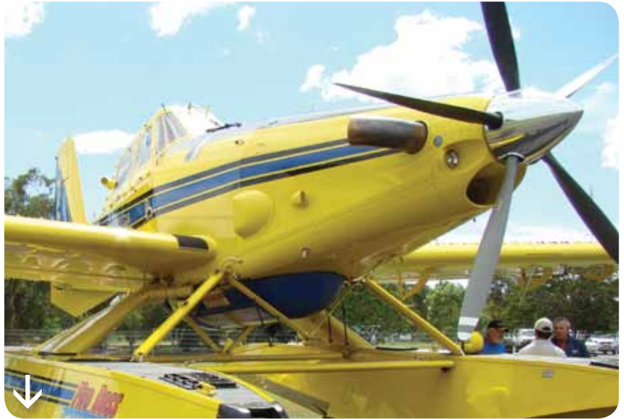
Plate 21. Shows the new Engine Ram Air Inlet located under the front spinner. Note also the Vortex generators added to the wing spar upper surface leading edges, a series of small vertical finlets.
