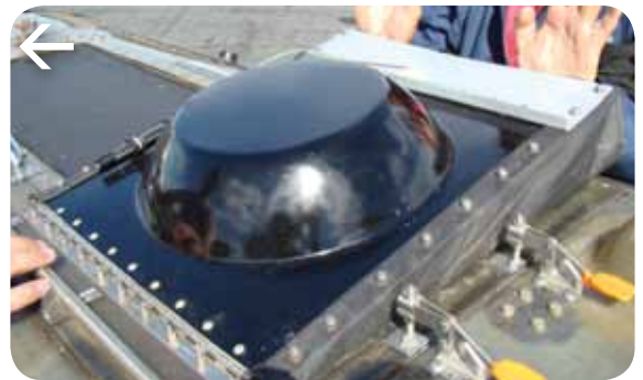
Plate 20. Shows the upper relief valve door.
