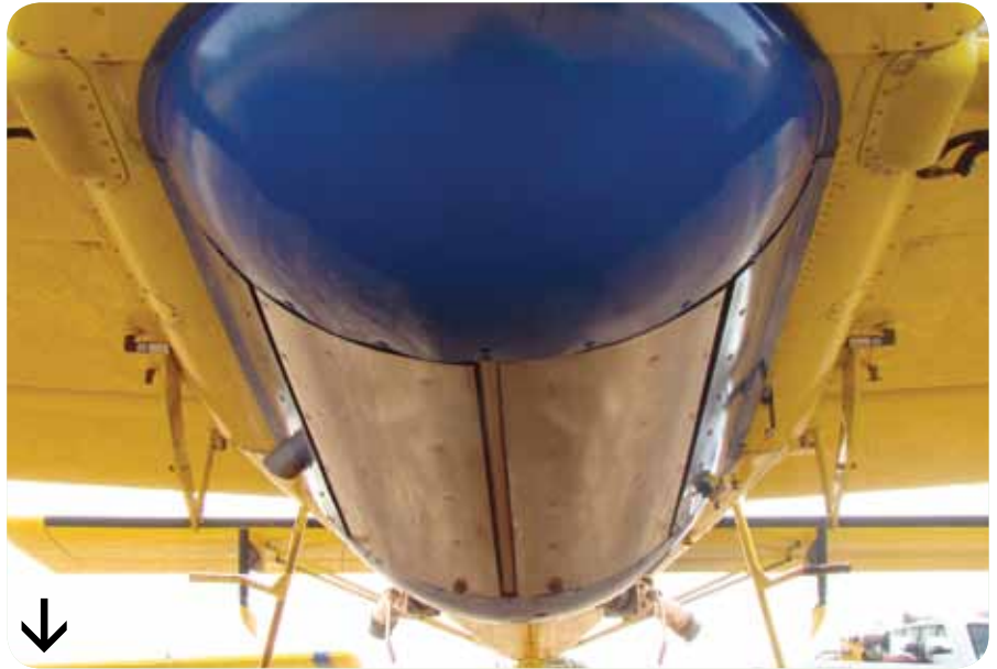
Plate 9. The FRDS longitudinal doors in the closed position.
