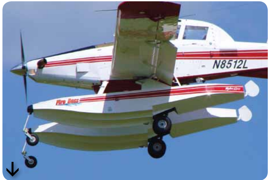
Plate 14. View of the Wipline amphibious floats and the retractable wheeled landing gear. Left side of image shows, the retractable nose mounted wheels and centre of image the retractable dual main wheels.
