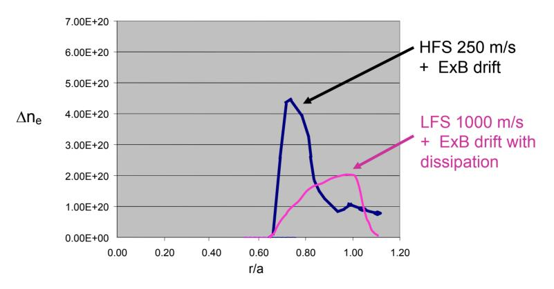
The resulting deposition from a 4 mm pellet injected from the outside midplane (LFS) and inner wall (HFS) including ExB drift effects to NGS pellet ablation. The calculation uses the Pellet Relaxation Lagrangian code to model the cloudlet displacement from ExB drift. Dissipation is ad hoc scaled from DIII-D results.
