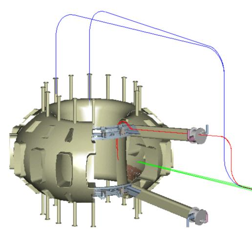
• Pellet speed limited to about 250 m/s for curved guide tubes for HFS launch
