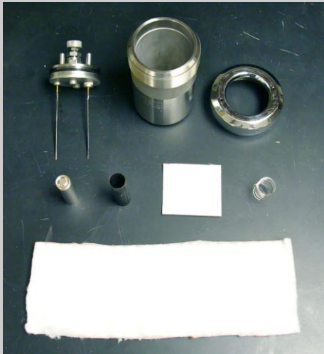
Bomb and other components for 18650 battery tests
