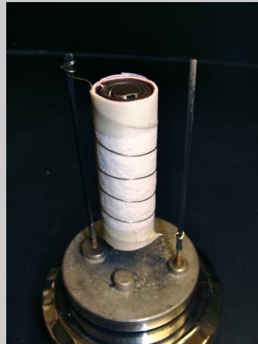
Bomb and other components for 18650 battery tests
