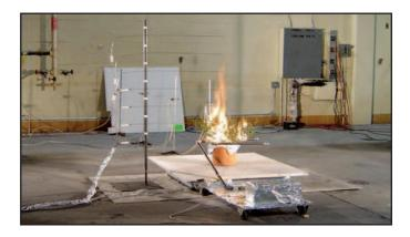
FIGURE 1: Controlled burn tests of shrubs were conducted at the National Institute of Standards and Technology.
