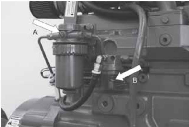
Fig. 43 Venting the fuel system on the fuel filter
