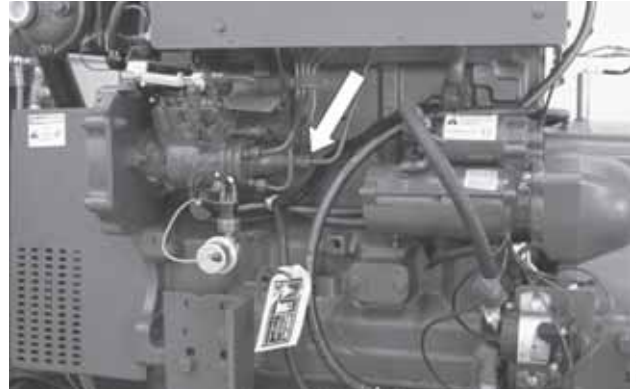
Fig. 44 Vent the fuel system on the diesel injection pump
