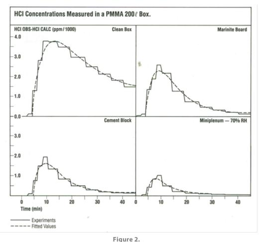
HCI from Thermal Decomposition of PVC Cables in a Lined PMMA Box
