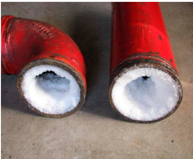
Photo 9: Ice plugs are a major problem in dry pipe systems, especially in freezer systems. Ice restricts the flow of water, can plug pipes and can prevent the sprinkler system from operating properly. NFPA 25 requires freezers to be inspected annually for ice plugs, and some companies perform this inspection at more frequent intervals. This ice plug was discovered using ultrasonic scanning. Used with permission.
