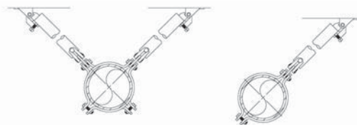
4-Way Riser Brace (Plan view)
