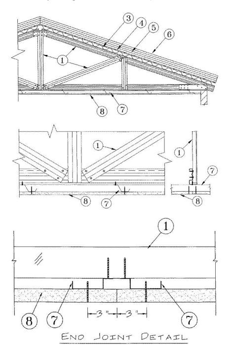
1. **Structural Steel Members\*** — Pre-fabricated light gauge steel truss system consisting of cold-formed, galvanized steel chord and web sections. Trusses fabricated in various sizes, depths, and from various steel thickness. Trusses spaced a max of 48 in. OC.
