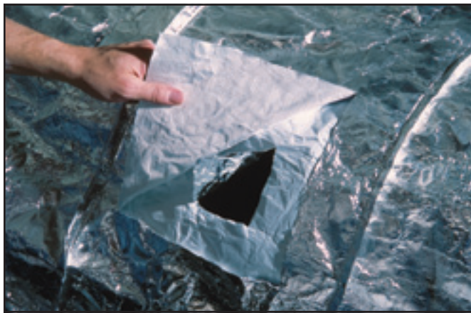
Figure 2—Fire shelters have two layers—the outer layer is silica laminated to aluminum foil, the inner layer is fiberglass laminated to aluminum foil.
