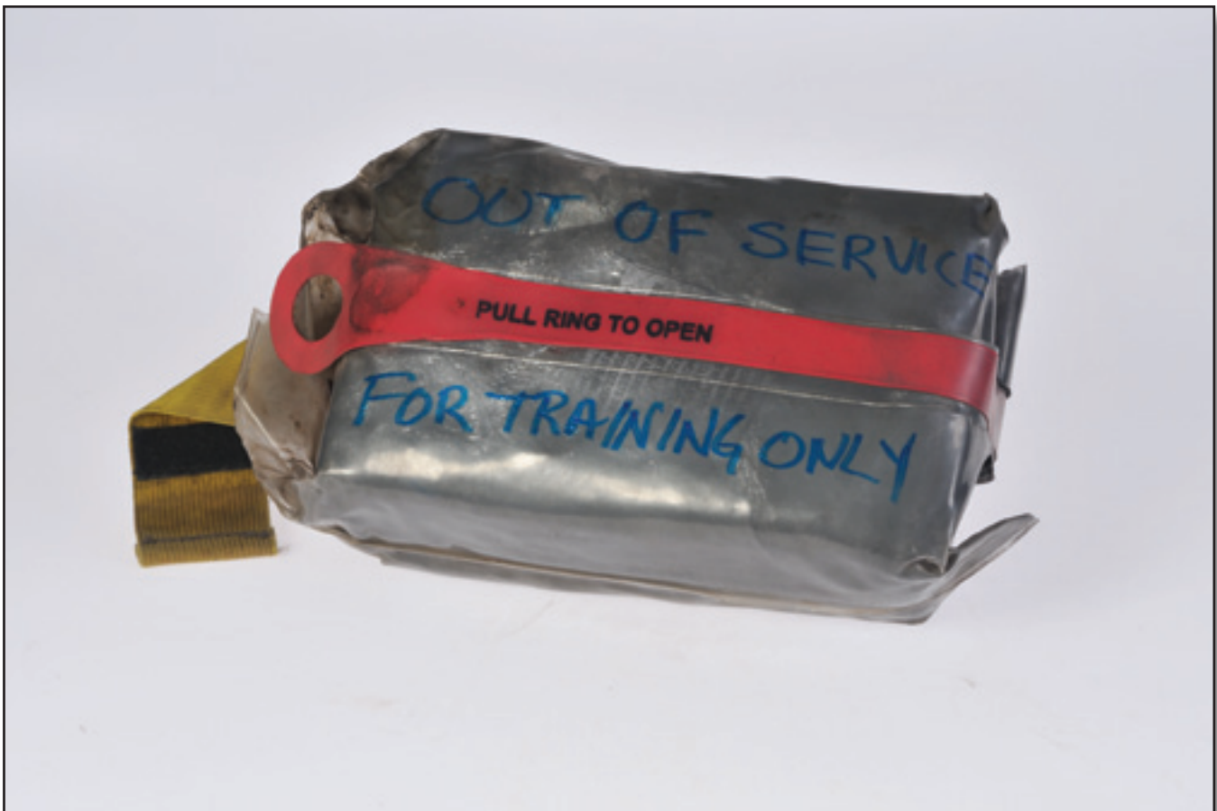
Figure 3—Mark fire shelters that are taken out of service to identify them as training shelters for practice deployments.
