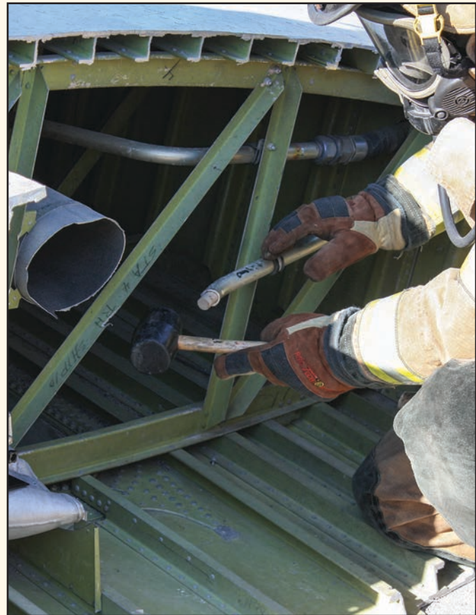
Step 3: Insert plug/plugging material into fuel line or hole in tank until leak stops.
