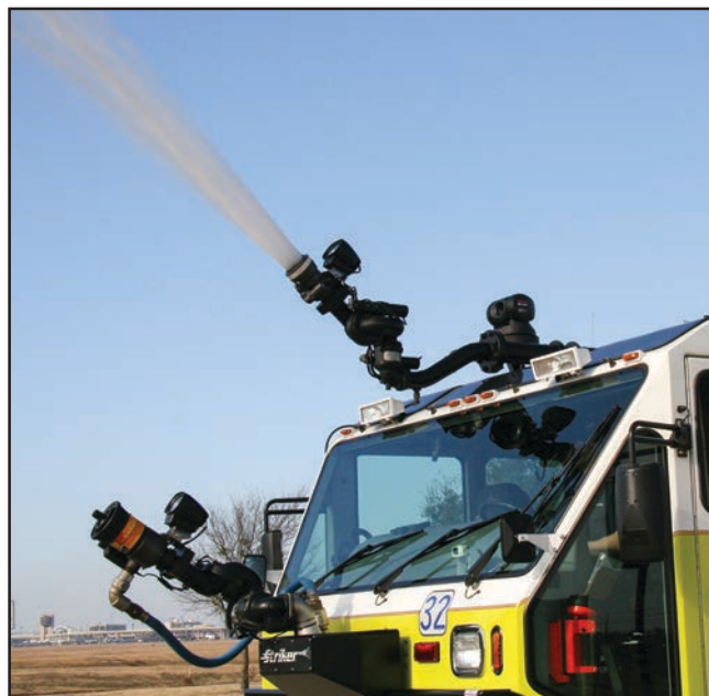
Figure 9.13 Examples of roof and bumper turret nozzles.
