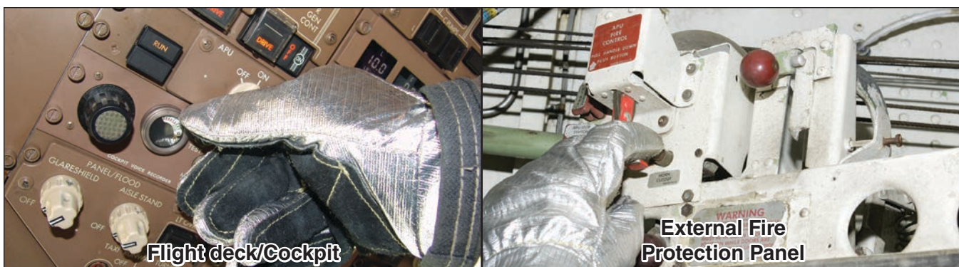
Figure 9.17 APU/EPU shutdown procedures can be accomplished from the flight deck/cockpit or an external fire protection panel. External image courtesy of Doddy Photography.
