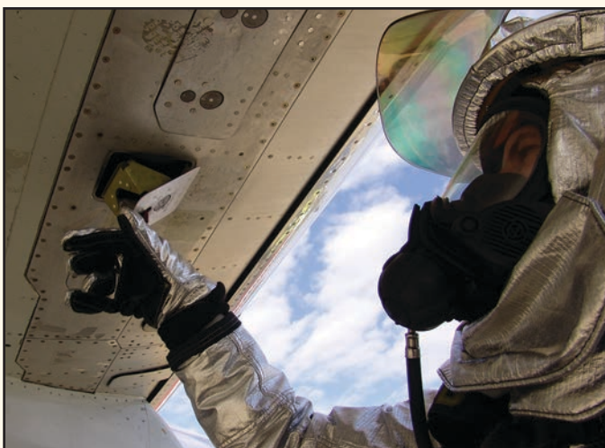
Step 2: Gain access to fuel valve for that line.
