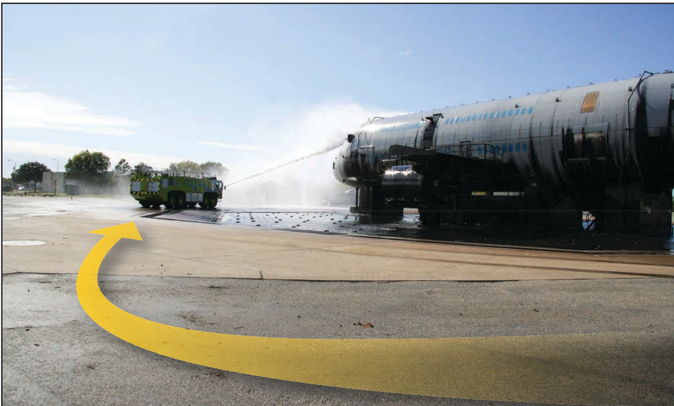
Figure 9.12 An ARFF apparatus pumping and rolling as it discharges agent.
