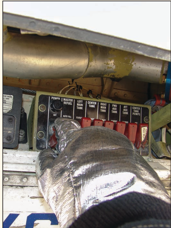
Step 3: De-energize fuel pump controls.
