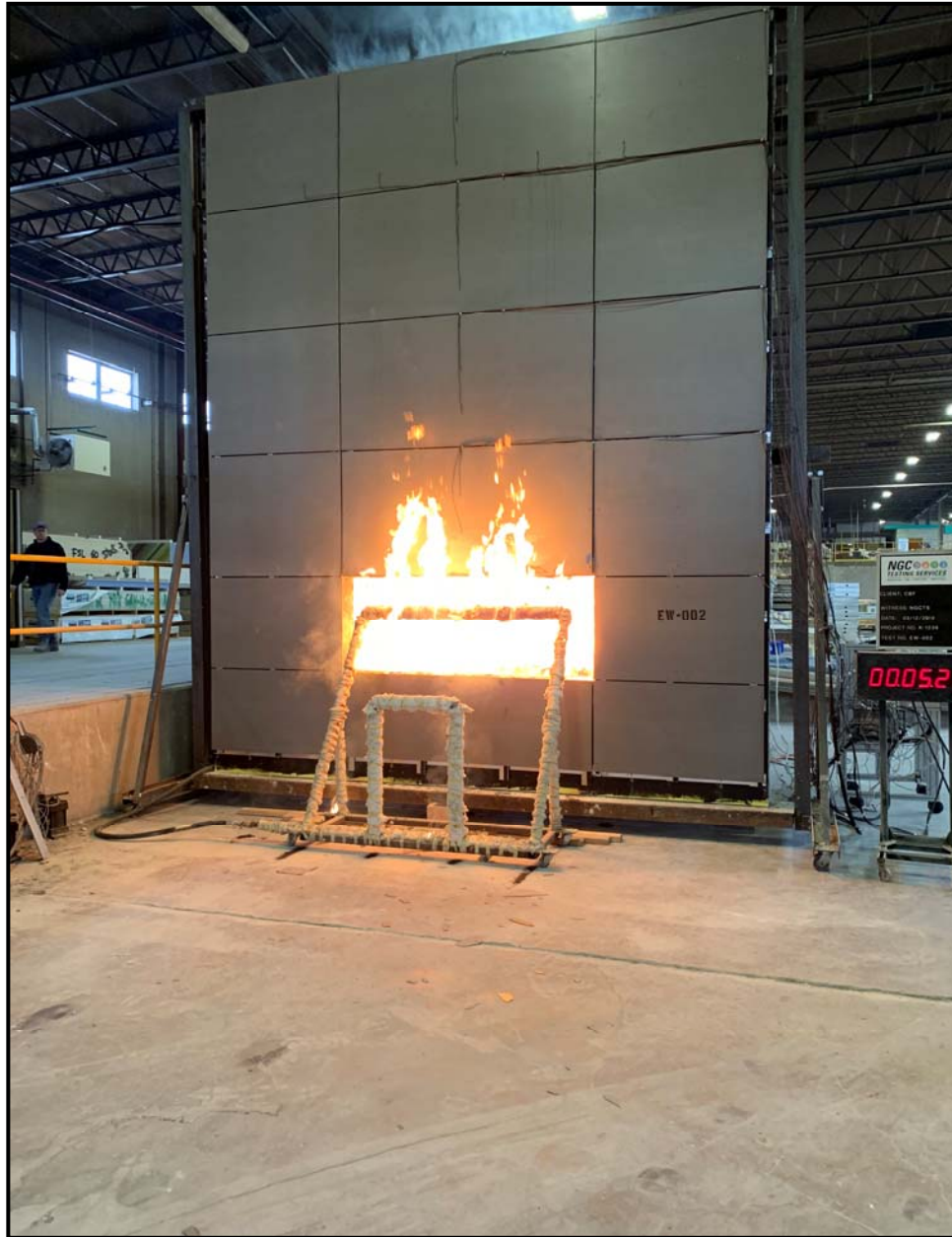
Photo 2: Test Specimen after Ignition of Window Burner
