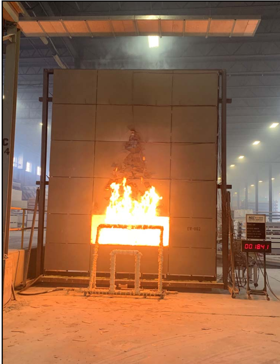
Photo 3: Cracking and Spalling of SILBONIT Panels
