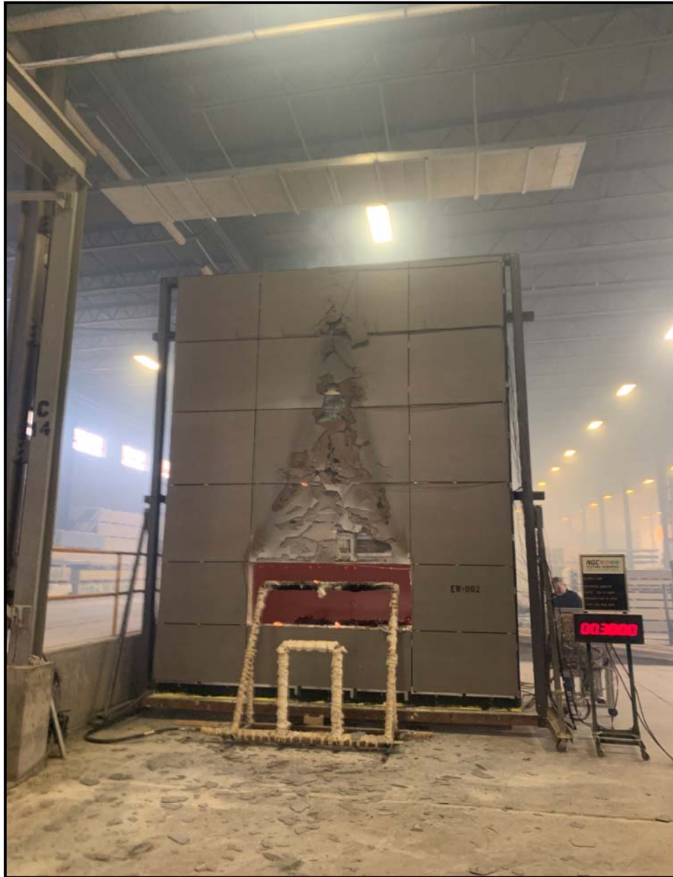
Photo 4: Test Specimen After Burners Extinguished
