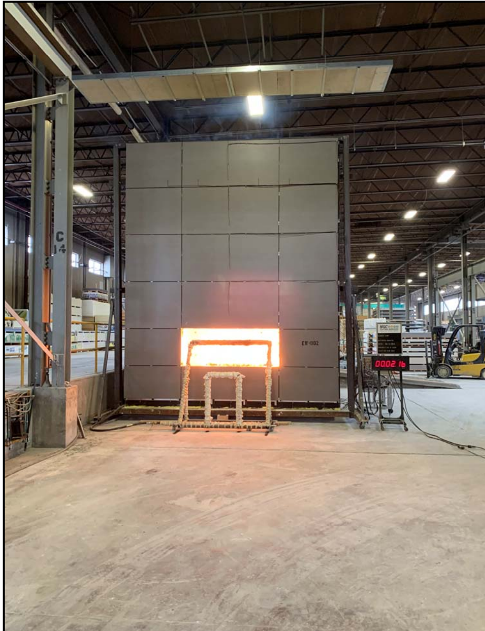
Photo 1: Test Specimen After Ignition of Room Burner
