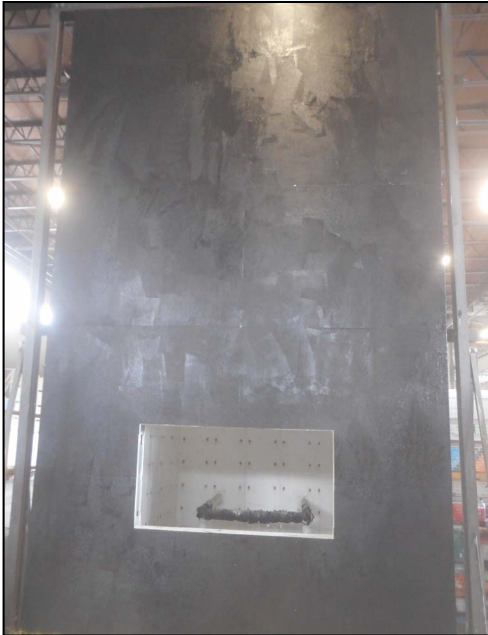
Photo 2: GE Elemax* 2600 AWB Applied to Exterior Sheathing
