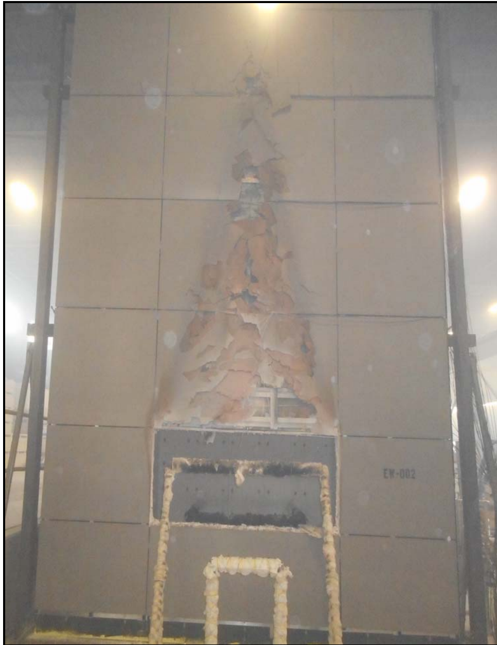
Photo 5: "Burn" Pattern of SILBONIT Panels
