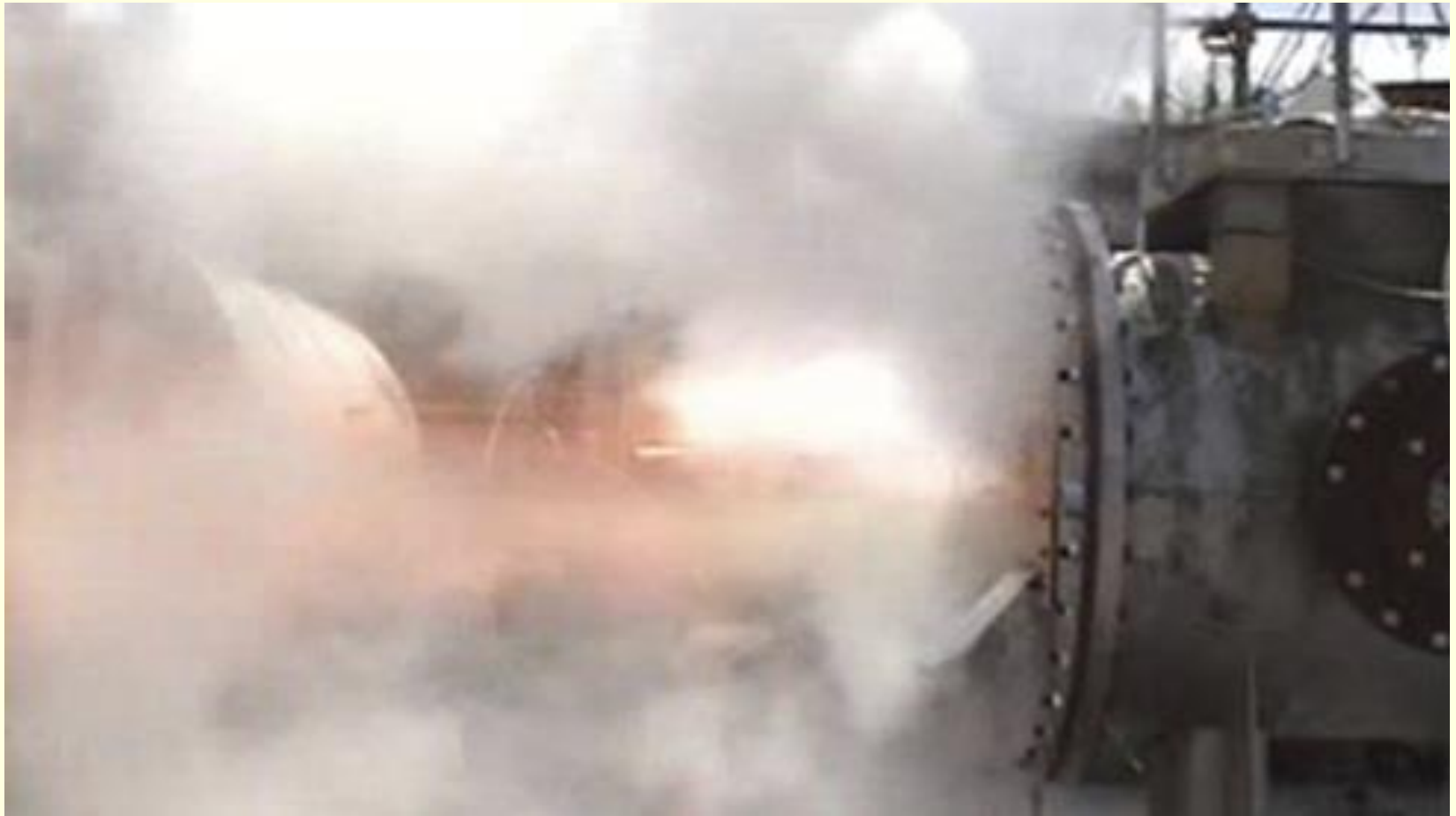
Corn Flour Explosion with Relief Venting
