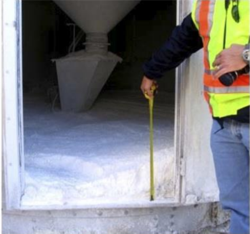
Cornstarch accumulation under cornstarch silo
