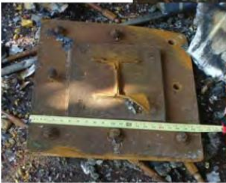
Support Column Sheared Off Baseplate
