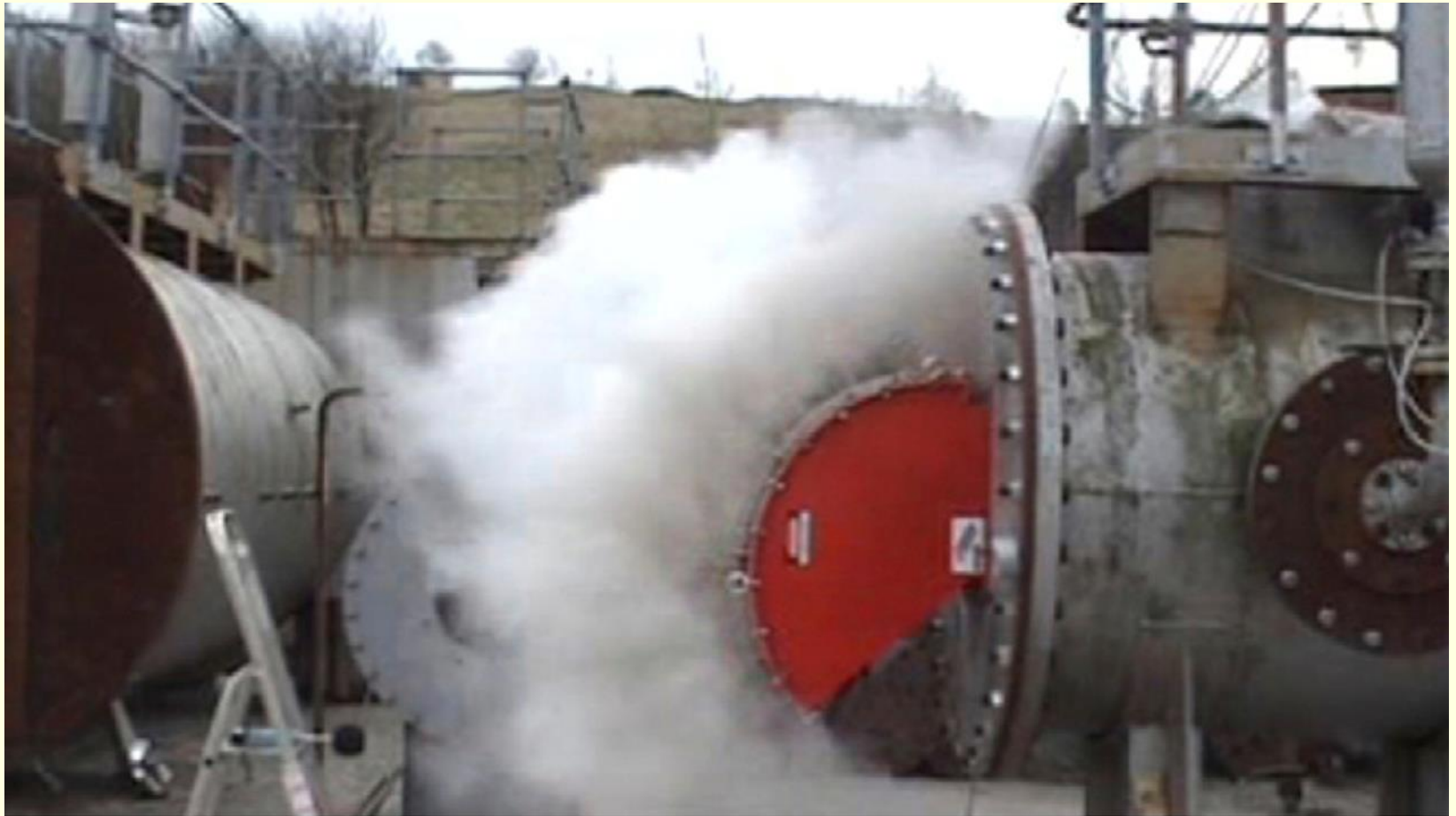
Corn Flour Explosion with Flameless Venting
