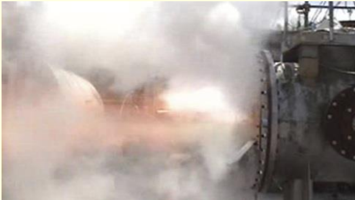
Corn Flour Explosion with Relief Venting
