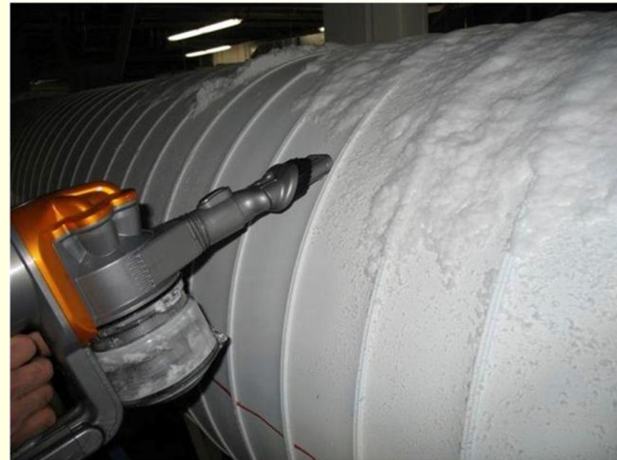
Dust Collection to Measure Accumulation
