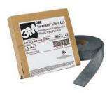
Graphite-based, largely inorganic, flexible, fire resistive, intumescent wrap designed to firestop plastic pipe penetrations in fire-rated walls, floors and floor/ceiling assemblies.
