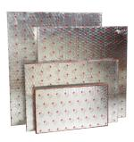
Intumescent sheet used to firestop large openings with applications including blank openings, through penetrations of multiple cable, pipe ducts, bus ducts and cable trays. Bonded on one side to a layer of 28-gauge galvanized steel.
