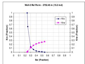
Figure 4 – Rel Perm Curves from SCAL experiments in Well Beta-5
