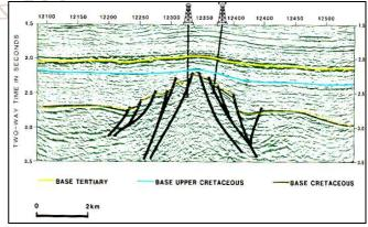
Figure 1 - Seismic Cross Section.
