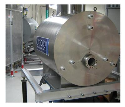
Figure 4.20: Image of the SIPT magnet before the beam line components for testing the MiniTrap had been installed.
