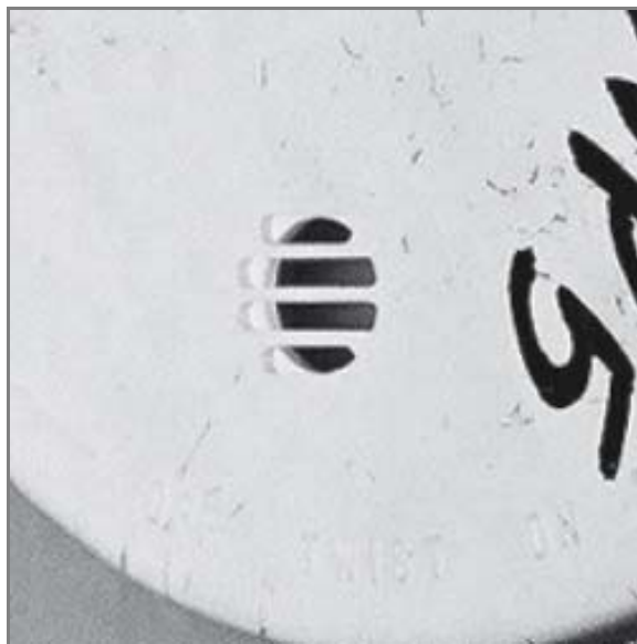
Figure 6.2.10.3(c) A Duplicate Powered (Functioning) Smoke Alarm After Exposure to the Same Sooty Atmosphere as the Smoke Alarm in Figure 6.2.10.3(a) and Figure 6.2.10.3(b), Displaying Typical Enhanced Soot Deposition.
