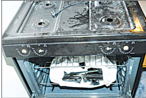
Figure 26.2.3(b) Gas Control Shafts in the OFF Position.
