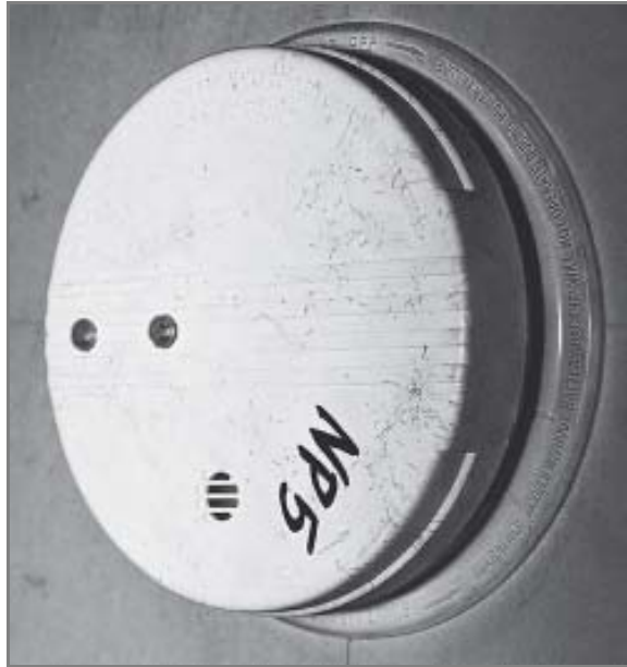
Figure 6.2.10.3(b) Close-Up Close-up of the External “Horn” (or Sound) Outlet of the Unpowered Smoke Alarm Displayed in Figure 6.2.10.3(a) After Exposure to a Sooty Atmosphere, Showing No Enhanced Soot Deposition.
