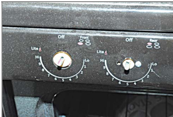
Figure 26.2.3(c) Gas Control Shaft with Ruler Depicting Control in the ON Position.
