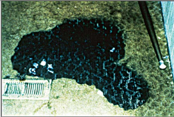
Figure 6.3.7.8.3(e) Test Burn on Vinyl Tiles.
