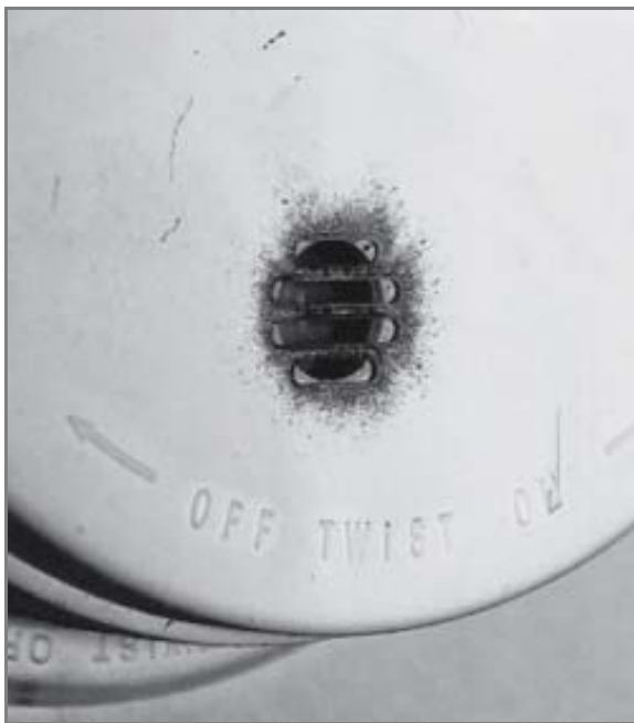
Figure 6.2.10.3(d) Close-Up Close-up of the External “Horn” (or Sound) Outlet of the Powered Smoke Alarm Displayed in Figure 6.2.10.3(c) After Exposure to a Sooty Atmosphere, Showing Enhanced Soot Deposition.
