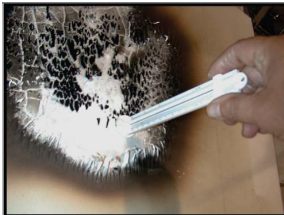
Figure 18.4.4.2(b) Measuring Depth of Calcination on a Piece of Gypsum Wallboard.
