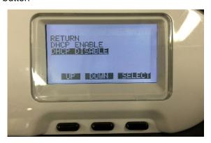
(7) Press the **UP** button until the **RETURN** is highlighted, then press the **SELECT** button
