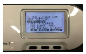
(8) Press the **DOWN** button until the **SET IP ADDRESS** is highlighted, then press the **SELECT** button
