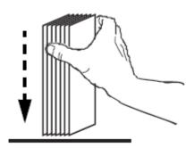
(3) Push the stack back and forth to an angle of about 45 degree from vertical, so as to separate all of the labels
