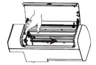
(6) Place the stack in the Feeder Cartridge in the correct orientation shown below.
