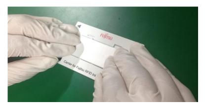
Snap the RFID Label in the cavity of the Reusable Carrier.
