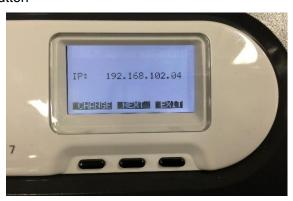
(9) Change to the assigned IP address using the **CHANGE** and the **NEXT** button, then press the **EXIT** button
