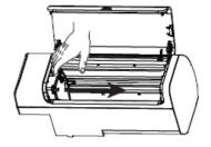
(3) Stick one of the sheet first to the bottom of the Feeder Cartridge aligning the sheet to the edge of the Feeder Cartridge as shown in the picture below with a red circle
