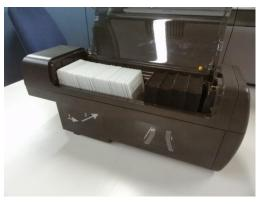
! Caution The Shock Absorber MUST be placed between the stack and the Card Stack Pusher
