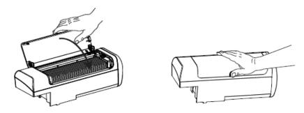
(8) Install the Feeder Cartridge by sliding it down and to the left into the receptacle. You will need to apply enough pressure for it to "snap" into place
