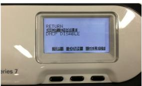
(6) Press the **DOWN** button until the **DHCP DISABLE** is highlighted, then press the **SELECT** button
