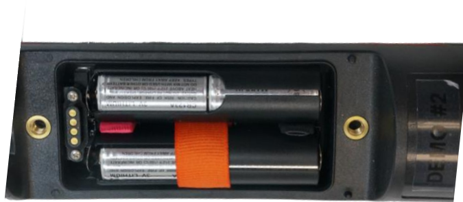
Figure 50: CR123A lithium batteries inside adapter tubes properly inserted into the FL360.
