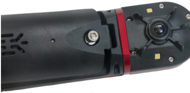
Figure 8: Align the Battery Lid with the camera housing.
