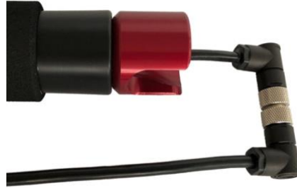
Figure 20: The right-angled cables route forward on the boom.
