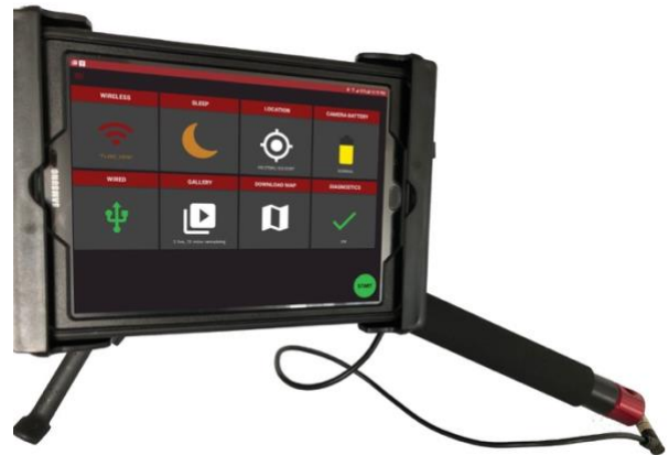
Figure 23: Tablet mounted onto the boom.
