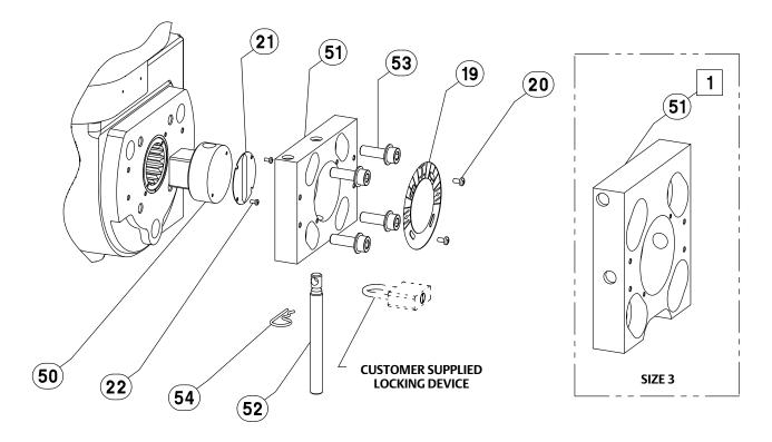
1 PART ORIENTATION FOR SIZE 3 END-MOUNT INSTRUMENT
