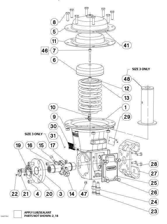
Figure 8. Fisher 2052 Size 3 Actuator Assembly
