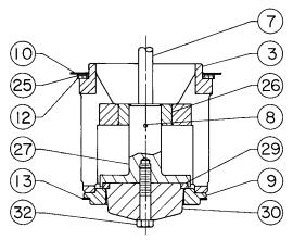
**EQUAL PERCENTAGE VALVE PLUG** 76.2 mm AND 101.6 mm (3 INCH AND 4 INCH) PORT DIAMETER
