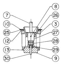
MICRO-FORM VALVE PLUG 6.4 AND 9.5 mm (0.25 AND 0.375 INCH) PORT DIAMETERS
