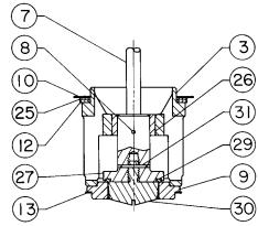
**EQUAL PERCENTAGE VALVE PLUG** 38.1 mm AND 50.8 mm (1.5 INCH AND 2 INCH) PORT DIÀMETER
