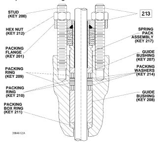
Figure 9. Typical ENVIRO-SEAL Packing System with Duplex Packing
