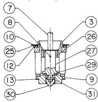
MICRO-FORM VALVE PLUG 12.7 mm THROUGH 25.4 mm (0.5 INCH THROUGH 1 INCH) PORT DIÀMETER
