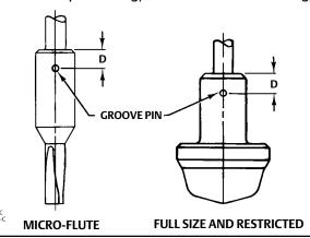
4. Place the stem/bellows assembly and valve plug or valve plug guide in a soft-jaw chuck or other type of vise so that the jaws grip a portion of the valve plug or valve plug guide that is not a seating or guiding surface. Drive out the pin (key 36, figure 11).
