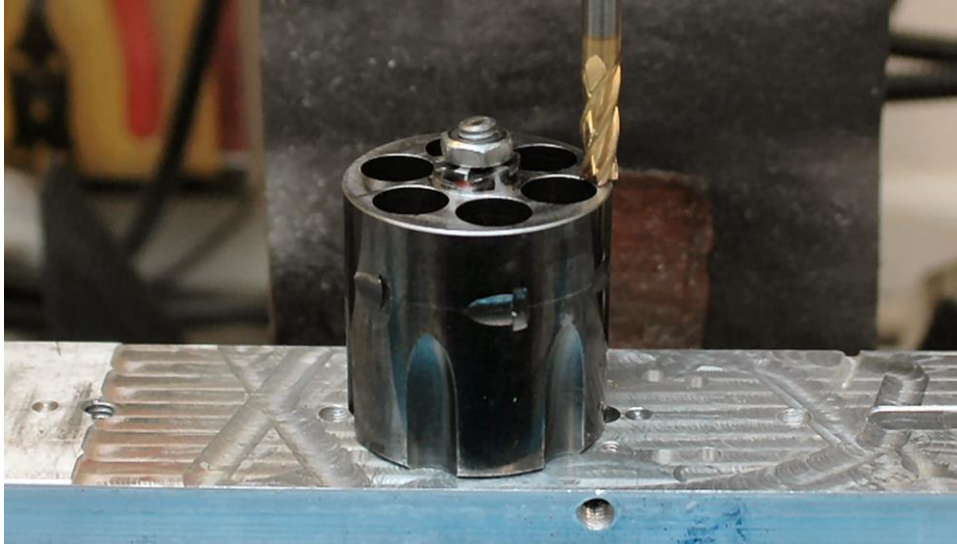
Figure 9: Milling Cylinder Face
