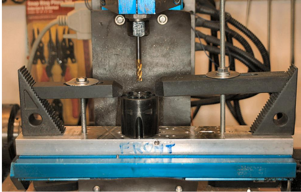
Figure 3: Setup for Milling the Ratchet
