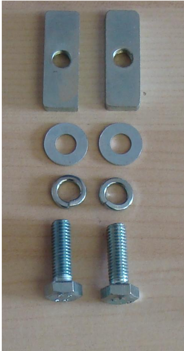
Bolts with plates welded on for mounting the Front Mounting Bracket.(See above)
