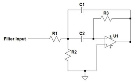
Figure 4: multiple-feedback bandpass filter
