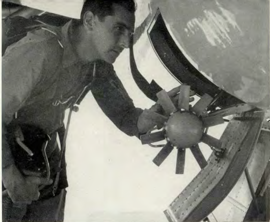
A handy gadget. The ram air turbine (R.A.T.) provides power for emergency hydraulic control.
