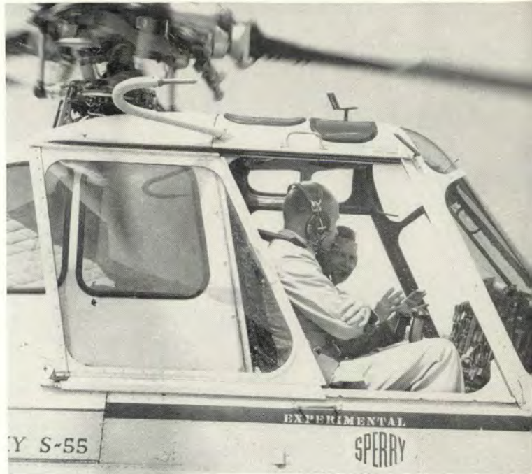
Above, new helicopter control system permits "hands off" flight. Below, pilot is freed for navigation duties. Light pattern on cyclic stick reveals movements required in 15 seconds of operation.
