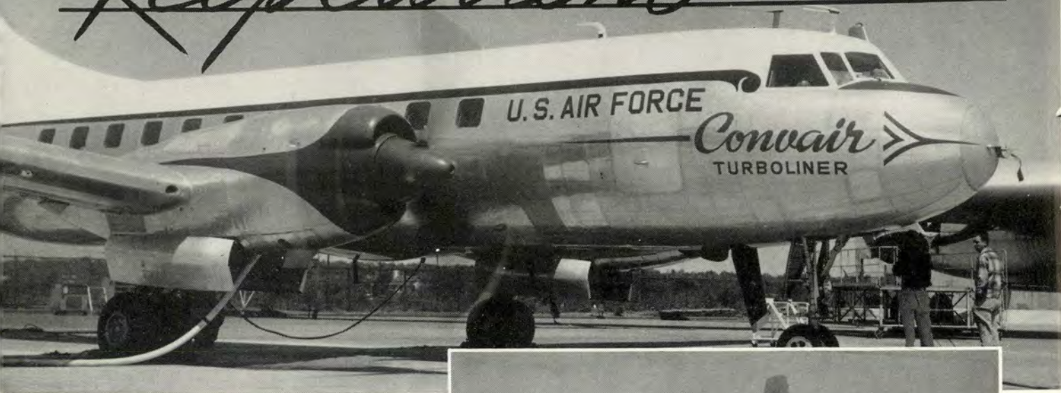
Note nacelles, above and right, on Convair YC-131C turboprop transport. It uses T-56 Allison engines.
