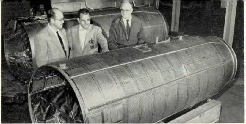
Dimpling of the entire surface of a new type of titanium shroud insulates engine from fuselage.
