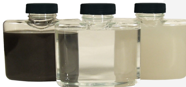
Left to right: dirty oil, clean oil, moisture-saturated oil
