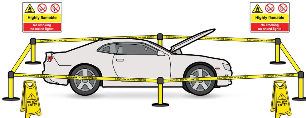
Appropriate fire CO2 or dry powder extinguishing equipment must be available.
