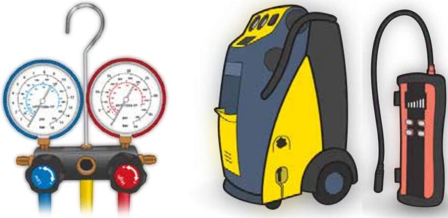
Only use equipment specifically designed for use with R1234yf refrigerant and complies with the relevant standards as shown in the table opposite.
