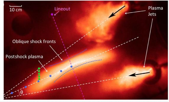
Fast-camera, visible-light image of two merging argon plasma jets, showing the formation of oblique, collisional plasma shocks.
