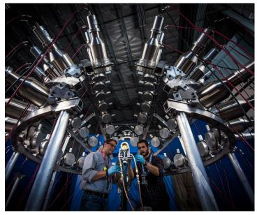
The Chi-Nu project is measuring the spectra of neutrons emitted from the neutron-induced fission of plutonium and uranium with emphasis on the low-energy and high-energy portions of the spectrum.
