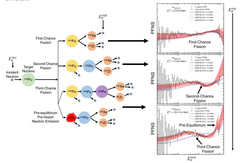
some cases. Pre-equilibrium, pre-fission neutron emission occurs in more energetic systems and changes the emitted neutron spectrum from fission as a function of detection angle. Neither this process nor its angle dependence had been observed for the neutron-induced fission of plutonium-239 and there were sparse data on this feature for uranium-235 before Chi-Nu.
