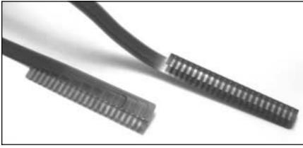
Pins can be inserted separately or ganged in a header. Minco recommends using a FR-4 or polyimide stiffener in pin areas to improve mechanical strength and simplify assembly.
