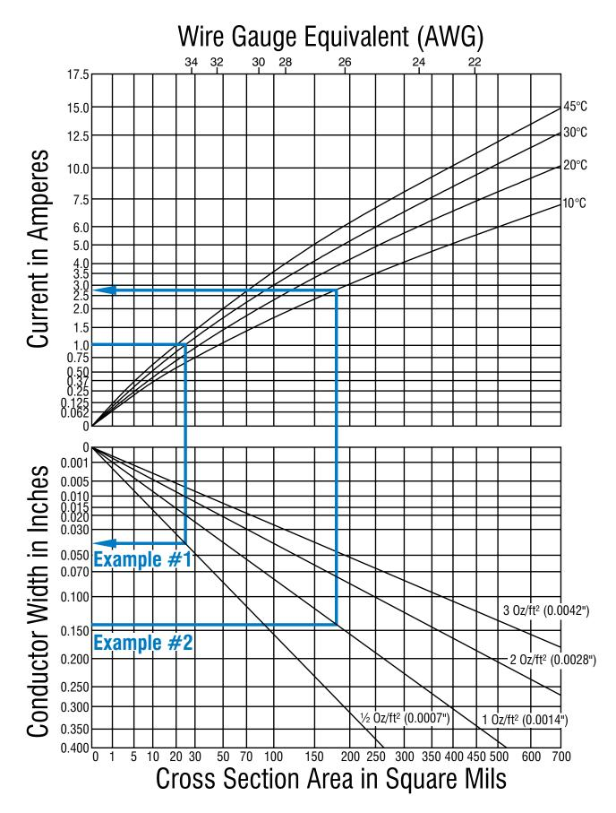
**Example #1**: A current of 1 amp with ½ oz. copper and 30°C temperature rise will require a conductor width of 0.040".
