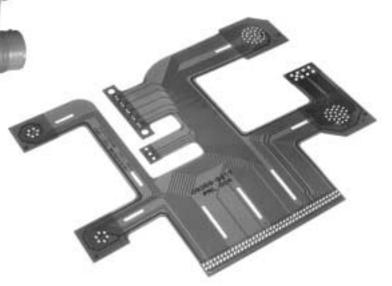
Commercial application – A flex-circuit with surface mount components folds to fit into a laser dimensioning device.
