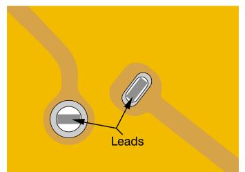
Round through-holes vs. slotted through-holes
