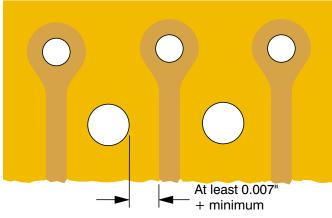
Non-wiring hole at least 0.007" + minimum from conductor.
