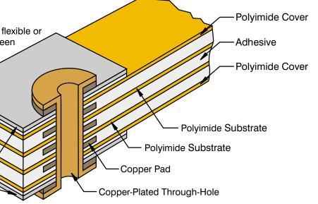
• Minco is capable of sequentially laminated, drilled, and plated circuits, which allows for more flexibility in designing the circuit.
