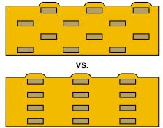
Staggered conductors vs. I-beam effect
