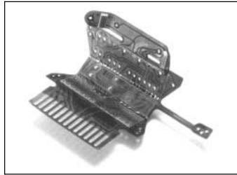
Small stiffeners used to force a bend line.
