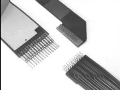
• Flex-circuits can interface to hardboards via soldered lap joints, lap joints applied with an anisotropic adhesive (conductive in the Z-axis only), compression dots using a raised metal dot, or 'zebra' strips. Compression methods usually require a stiffener behind the contact area.
