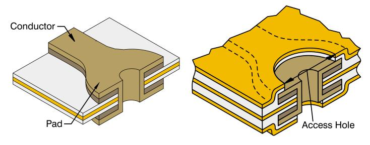
3. Copper is etched to create conductors and pads
