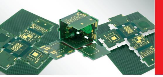
The trend to miniaturization in electronics continues. Integrated circuit board solutions are becoming more and more popular as a means of efficiently utilizing the even smaller casing volume in all three dimensions.
