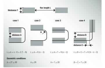
With short flexible areas, four bonded flex layers are easier to bend than 2+2 flex layers with airgap
