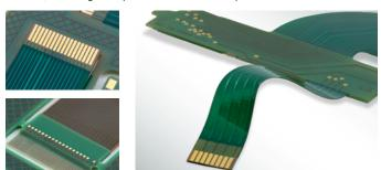
With flex-rigid and inner layer is flex, changing to outer layer by means of vias near to the ZIF area is recommended
