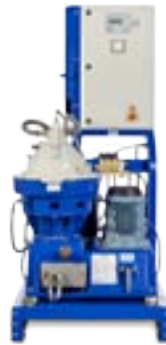
SINGLE FLEX MODULE with separator (excluding heater and pump)
